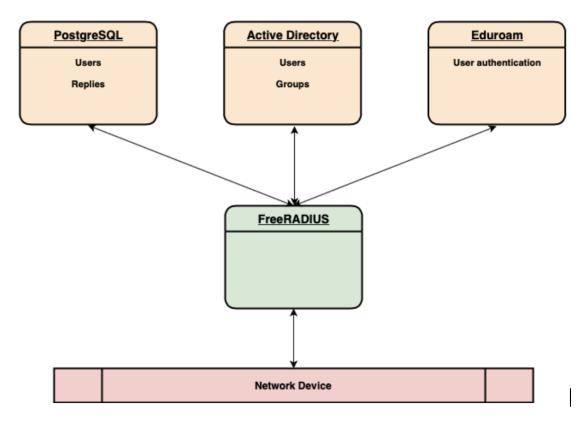
The network device will communicate with FreeRADIUS, which will determine if it should try to find the user in the local SQL database, do a lookup in AD or act like a proxy and forward the request to Eduroam. If we are going to use AD, we will first authorise the user with NTLM and in a second step use LDAP to lookup which groups the user belong to and based on that assing VLANs etc.
